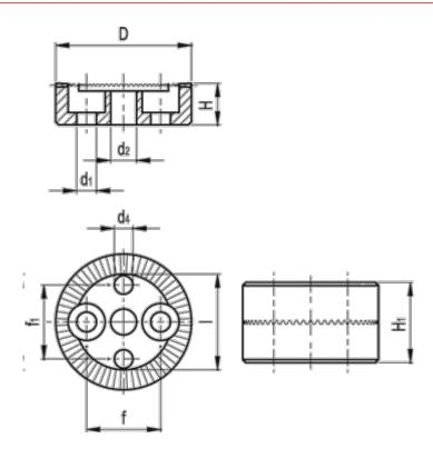
$$\begin{array}{lll} D & = 22 \\ d & = M4 \\ d1 & = 3.2 \\ d4 & H11 & = 3 \\ f & = 12 \\ f1 & = 12 \\ H & +/-0.9 & = 6.5 \\ H1 & = 13 \end{array}$$
